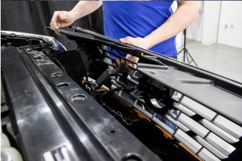
6. Carefully dismantle the radiator grille by unlatching the latches at the bottom.
