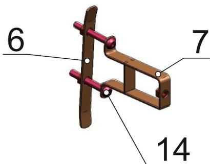
32. Install the number embedded parts (pos. 6 and 7) onto the bumper grille using screws M6x50 (pos. 13).
