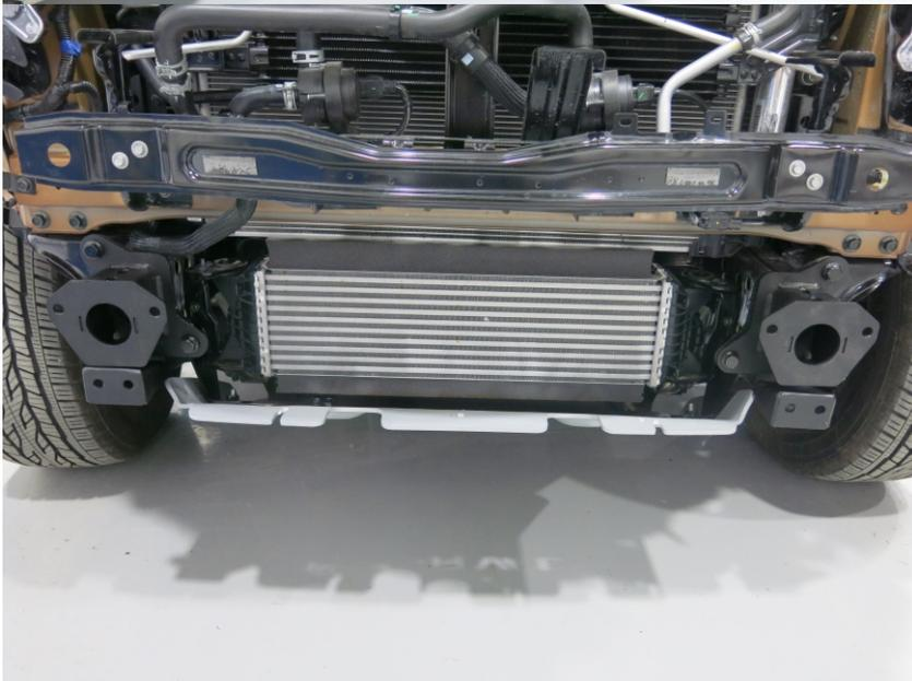
24. Install adapters (pos. 4 and 5) onto the vehicle frame using standard fasteners from the frame booster. Do not tighten screw joints.
