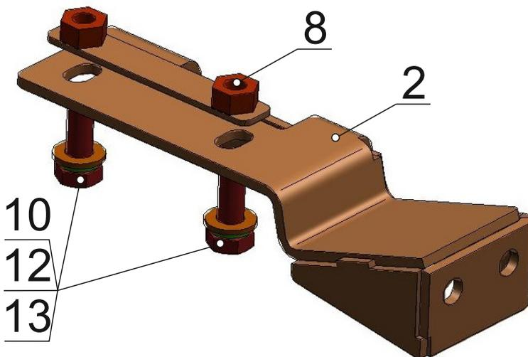
22. Install left frame booster (pos. 2) onto the vehicle frame and secure it to embedded part M12 (pos. 8), bolts M12x1,25x40 (pos. 10) and washers (pos. 12). Do not tighten screw joints.
