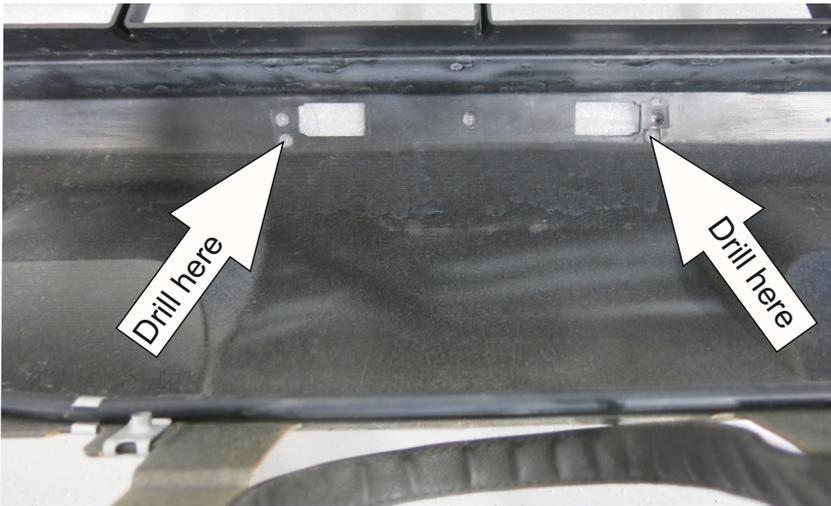
26. Temporarily install standard bumper for pad eye hole spacing. Mark the hole for pad eye fasteners on the inside of the bumper along the winch bracket.
