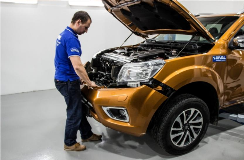
13. Dismantle the bumper. Pull the bumper edge by unlatching the latches, moving from the bumper edge to the center.
