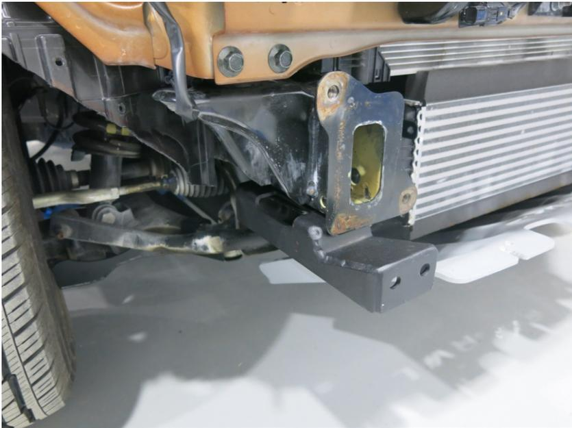
23. Install right frame booster (pos. 3) onto the vehicle frame, secure with standard bolts with installation of standard towing eye. Do not tighten screw joints.
