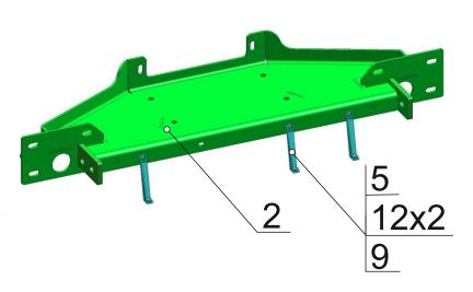
10. Install bumper brackets (2) to winch bracket (1) using bolts M6x20 (5), nuts M6 (9) and washers (12).
