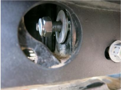
14. Fix winch bracket using bolts M12x40 (7), nuts M12 (11), washers (15 and 17).
