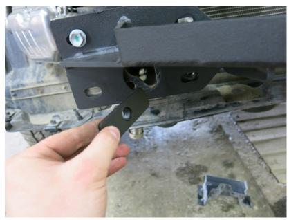
13. Fix winch bracket to insert nut M12 (4). Place insert nut into hole in the chassis and fix it using bolt M12x40 (7), washers (15 and 16).
