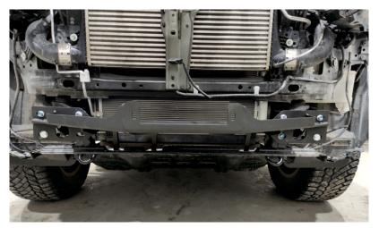
11. Install winch bracket (1) to the chassis using factory bolts, bolts M10x40 (6), nuts M10 (10) and washers (14).
