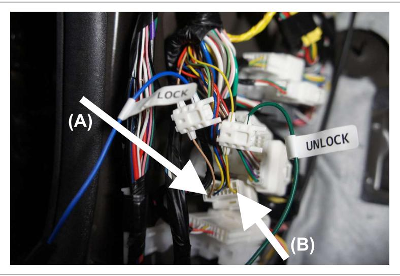
(B) Locate the YELLOW cable(1st down on right). Pale GREEN canopy cable "UNLOCK" using the scotch lock as shown.
