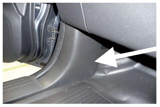
On RG-01 D-Max, remove the LHS kick panel under the steering-wheel.
