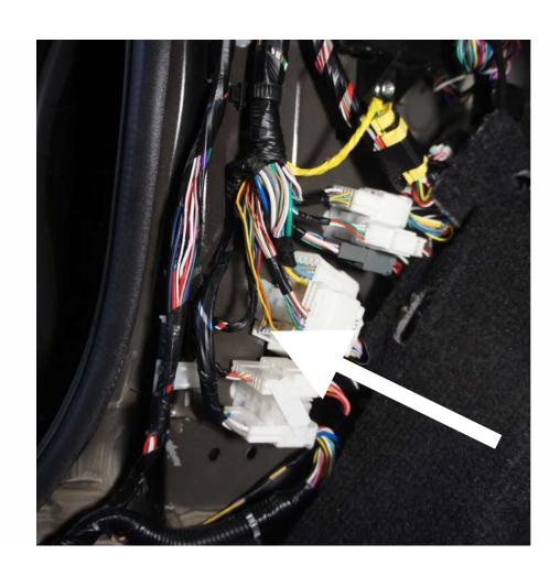
(A) Locate the LIGHT BROWN cable(1st down on left). Pale BLUE canopy cable "LOCK" using the scotch lock as shown.
