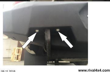
8. Install the bumper facia (pos. 1) onto the bracket and secure it in the towing eye area using screws M10x30 (pos. 7) and washers 10 (pos. 9).
