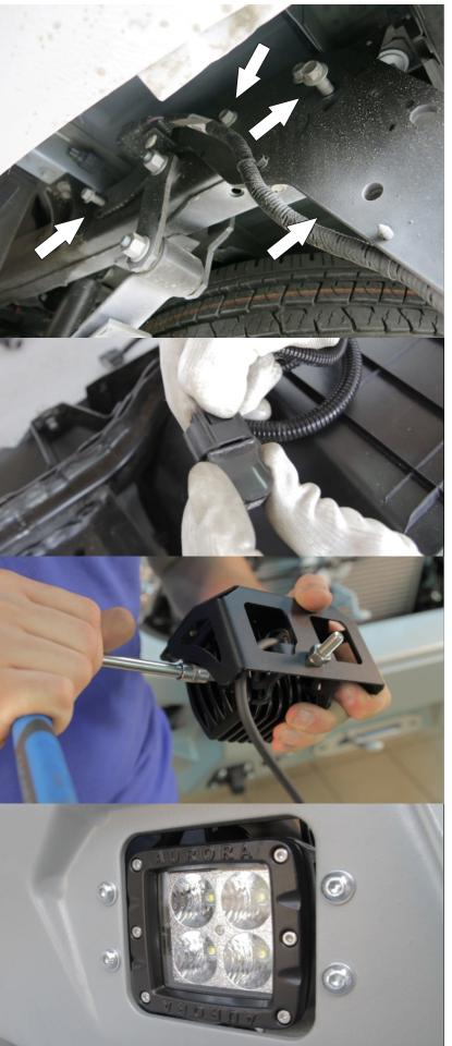
1. Unscrew tension bolts of the standard under-run bar the left and right of the vehicle frame. Dismantle the bumper.
