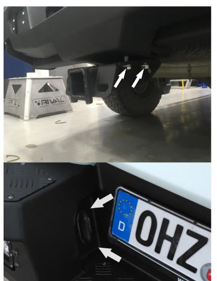
9. Install the tow bar square using bolts M12x40 (pos.11) and washers 12 (pos.12) on two sides. Tighten all screw joints.
